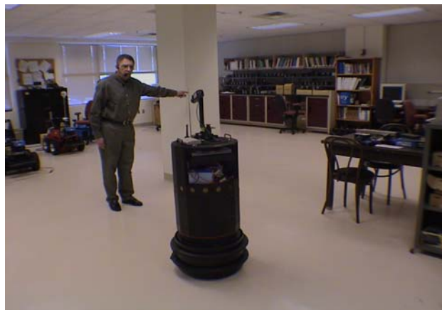
Fig. A.2. A human user indicates a distance manually with the utterance “Coyote, back up this far.”
