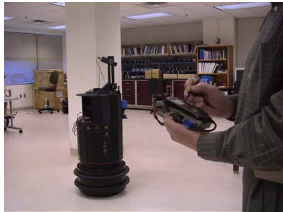
Fig. B. A human user indicates a location using a Personal Digital Assistant.
