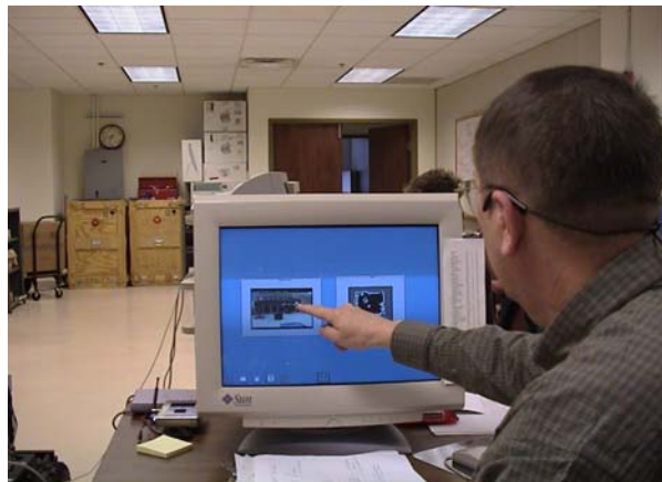
Fig. C. The human user, wearing a wireless microphone, interacts with a robot via a touch screen and speech.
