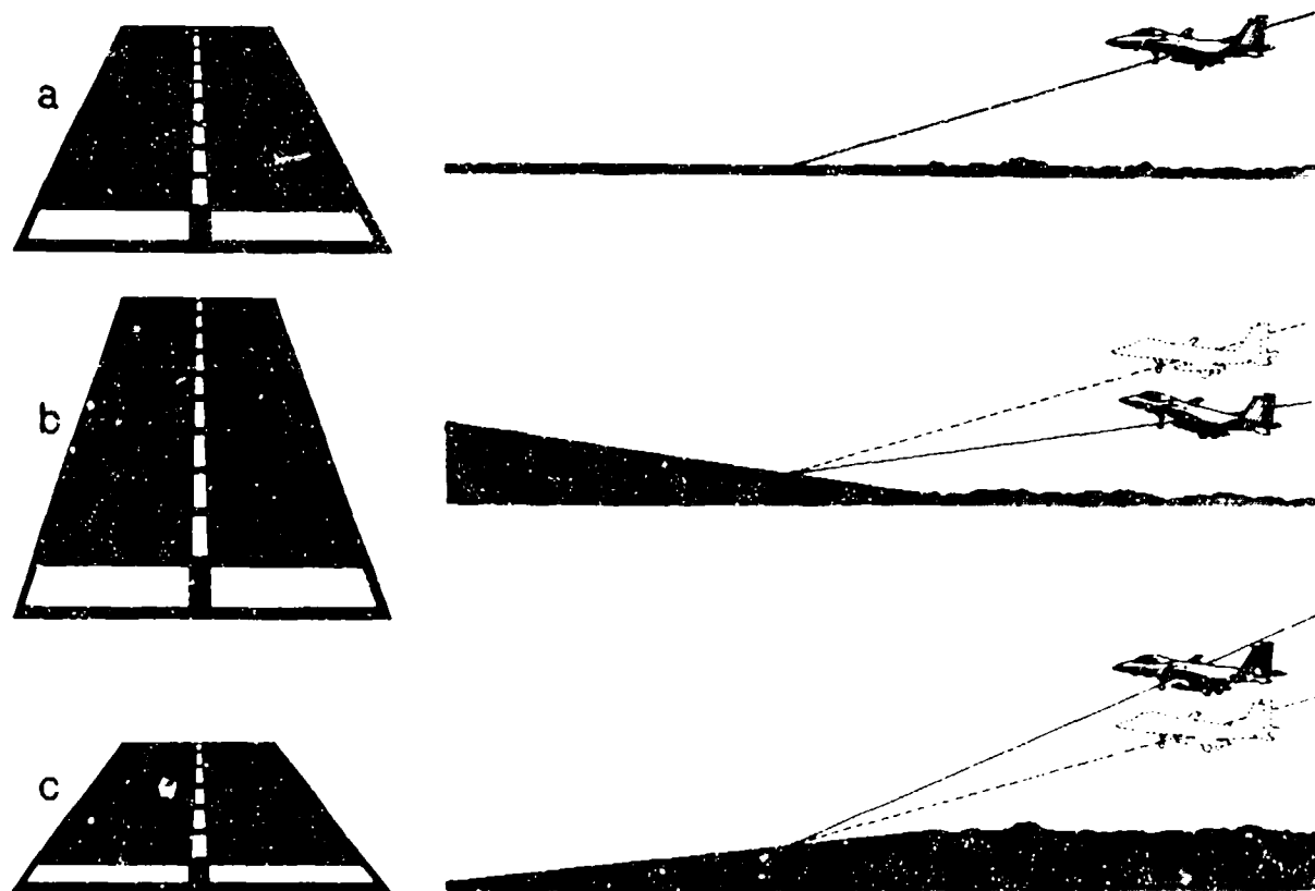
Figure 14. Effect of runway slope on the pilot's image of runway during final approach (left) and potential effect on the approach slope angle flown (right). a. Flat runway--normal approach. b. An upsloping runway creates the illusion of being high on approach--pilot flies the approach too low. c. A downsloping runway has the opposite effect.
