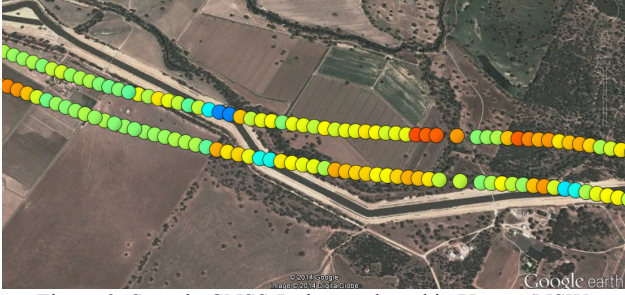
Figure 2. Sample GNSS-R data gathered in Yanco (NSW, Australia) from 1 km height. Note the reflectivity changes due to terrain inhomogeneity, and the large contrasts when coherent reflections occur over the irrigation water channel.
