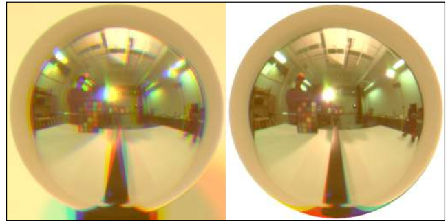
Fig. 6 An HDR image captured with the real time light probe before ( left ) and after ( right ) the alignment rotation of the color channels. The alignment works very well for most parts of the image. Only objects which are close to the mirror sphere and reflected near its edge will be slightly misaligned due to parallax.
