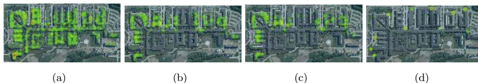
Figure 6: (a) Heat-maps representing all device positions; (b) Only inside to outside movements (leaving the building); (c) Positions of filtered exits; (d) Estimated exits constrained to real exits.
