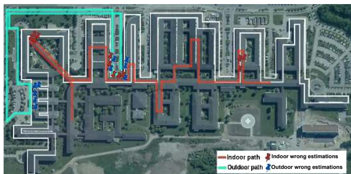
Figure 3: Geometry that defines the perimeter area of the building complex. Indoor and outdoor paths and examples of wrong estimation cases.
