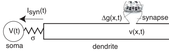
Figure 3. Schematic diagram of a neuron consisting of a soma resistively coupled to one end of a dendritic cable. A synaptic conductance change \Delta g(x, t) at position x on the cable induces a synaptic current into the soma at x = 0 .
