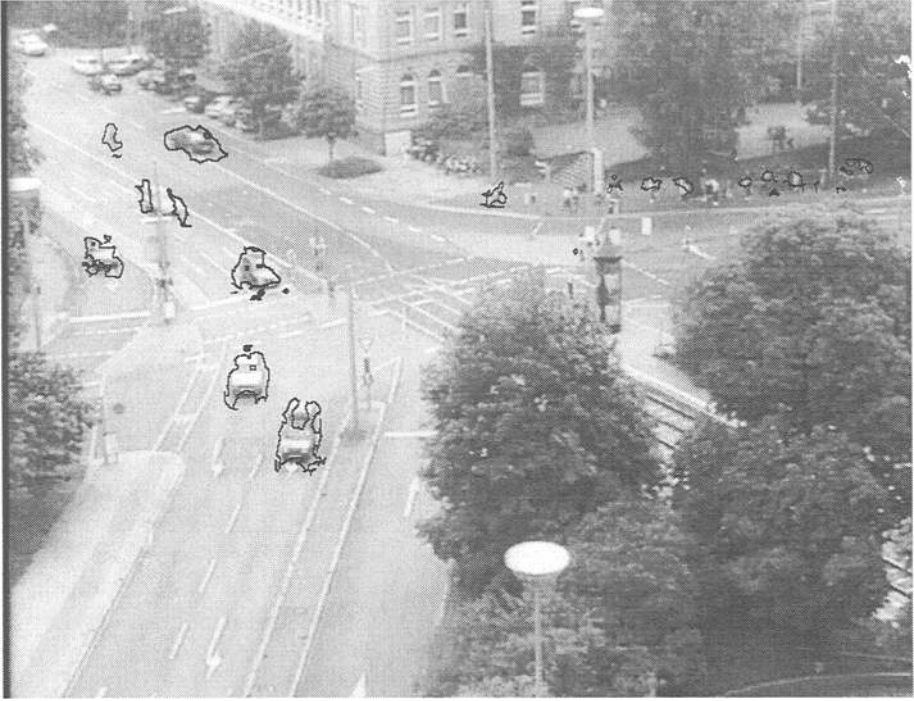
Fig. 6. Image frame as shown in Fig.1, with superimposed connected regions (indicated by their contour lines) determined according to the algorithm described in Sect. 6. The smaller masks in the top right quadrant as well as the one close to the top left corner correspond to moving people. Note the two masks around the top of a pole in the upper left quadrant: these two masks belong to a vehicle which is partially occluded by this pole.
