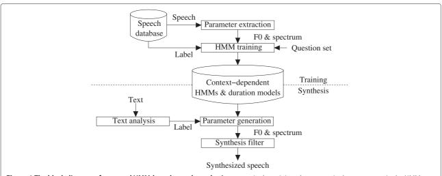
**Figure 1** The block diagram of a general HMM-based speech synthesis system. In the training phase we train the parameters in the HMMs given a labeled speech data set. In the synthesis phase, we use the model parameters to generate speech given text.
