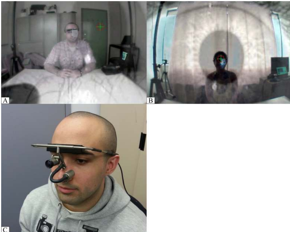
Fig 1. Dikablis eye tracker and associated video streams. Each Dikablis has a forward facing camera capturing a live video stream of the other participant, and the eye gaze of the wearer is overlaid on the video (A-B). Dikablis eye tracker worn by a participant (C). The individuals in this manuscript have given written informed consent (as outlined in PLOS consent form) to publish these case details.
