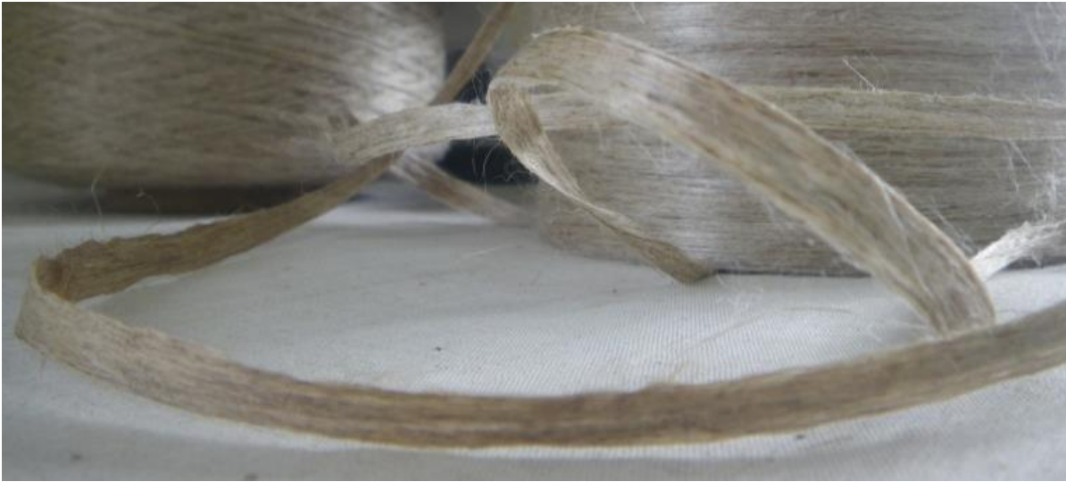
Figure 7. Flax yarn assembled by adhesive bonding
