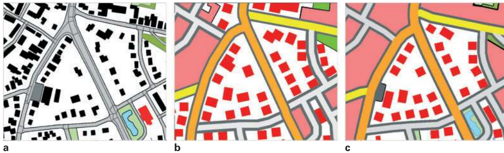
Figure 7. Optimally locating buildings in limited amount of space: (a) original buildings in TOP10NL, (b) buildings manually optimized by a cartographer, (c) buildings generated by the ESRI prototype Optimizer engine. Note that the rule to convert individual buildings to built-up area may have been applied differently in b and c
