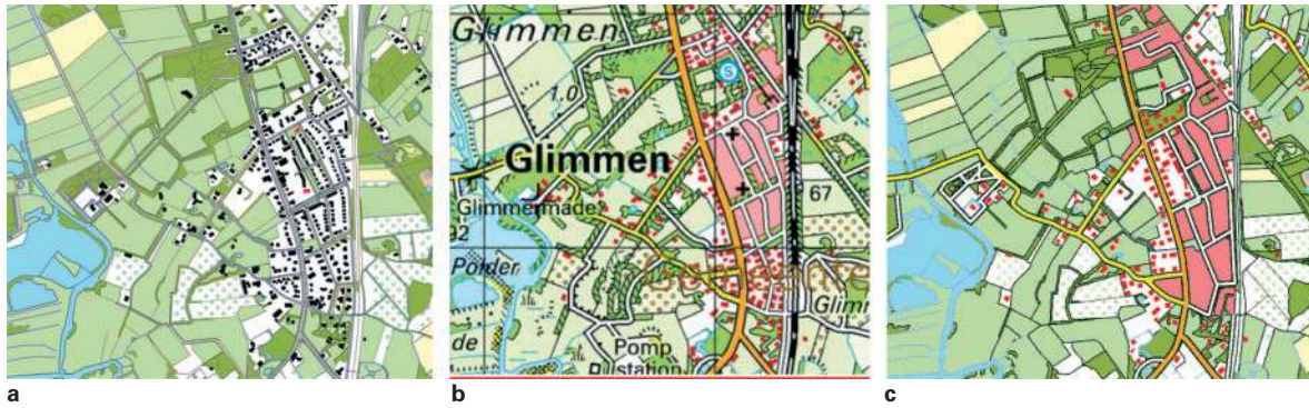
Figure 14. TOP10NL (left), interactively (middle) and automatically (right) generalized TOP50. Note that the automated solution only followed a selection of specifications as discussed in this paper and therefore, some basic operations (e.g. enlarging railways) were omitted
