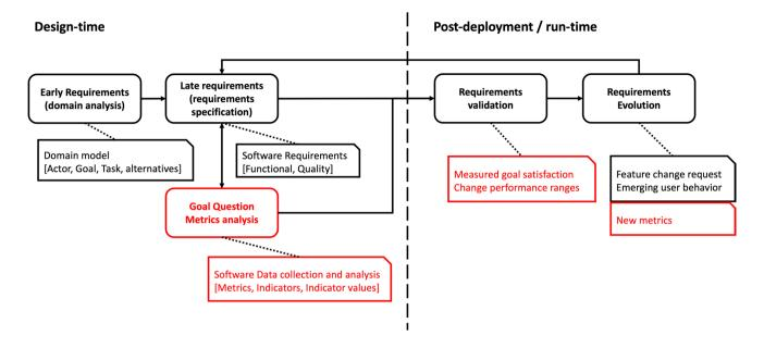
Fig. 4 The envisioned process with new tasks and artefacts highlighted in red
