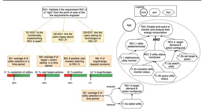
Fig. 2 Excerpt from the requirements model (right side). GQM applied to the requirement goal RG1.3 (left side). The connection between the measure M1 and the goal RG1.3 and the task T1.3a (at the bottom)
