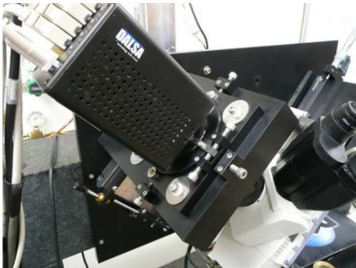
Figure 5. KESM camera and objective focusing controls.
