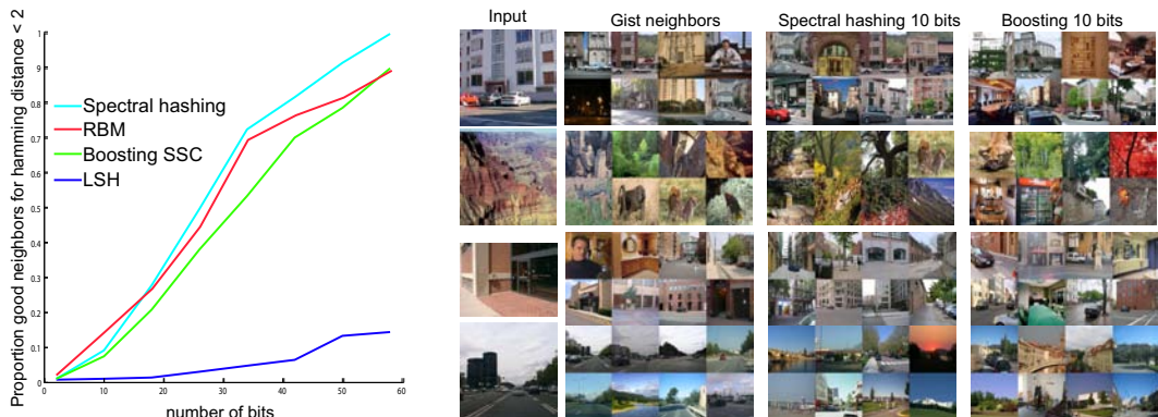
Figure 5: Performance of different binary codes on the LabelMe dataset described in [3]. The data is certainly not uniformly distributed, and yet spectral hashing gives better retrieval performance than boosting and LSH.
