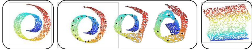
Figure 1.4 Intuition behind LLE. Left: n = 2000 input patterns sampled from a Swiss roll. Middle: results of minimizing of eq. (1.9) with k = 20 nearest neighbors and \ell = 25 , \ell = 15 , and \ell = 10 randomly chosen outputs (indicated by black landmarks) clamped to the locations of their corresponding inputs. Right: two dimensional representation obtained by minimizing eq. (1.9) with no outputs clamped to inputs, but subject to the centering and orthogonality constraints of LLE.
