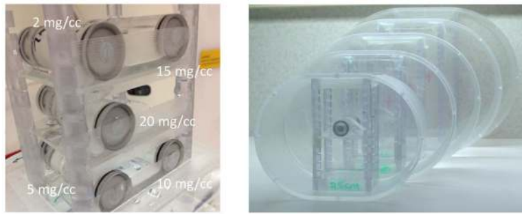
Figure 2. Vials containing different iodine solutions (left) were placed inside water phantoms representing patient torso with different sizes (right).
