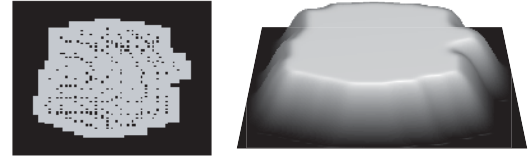
Figure 10: Blending function for the patch of Fig. 6. The left image shows the splatted interior sample points with black dots indicating the sample positions. On the right, the blending function after convolution filtering.
