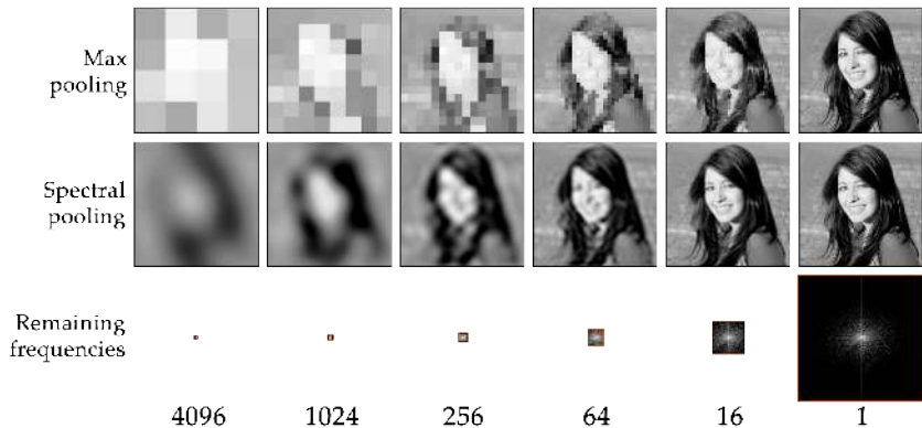
Figure 2: Approximations for different pooling schemes, for different factors of dimensionality reduction. Spectral pooling projects onto the Fourier basis and truncates it as desired. This retains significantly more information and permits the selection of any arbitrary output map dimensionality.
