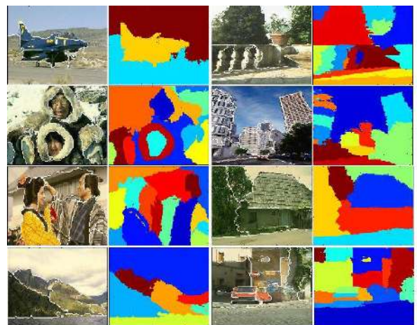
Figure 12: Multiscale Ncut prevents braking large uniform image regions into smaller parts due to its efficient use of long range graph connections.
