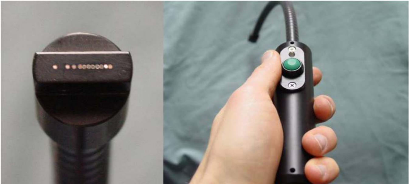
Figure 1. end-view of the optical probe used for reflectance and fluorescence measurements, and operator's-eye view showing the operator control.
