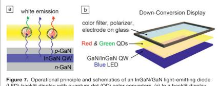
(LED)-backlit display with quantum dot (QD) color converters. (a) In a backlit display, blue emission from an InGaN/GaN quantum well (QW) LED is partially absorbed by green- and red-emitting QD down-converters; the mixture of three emitted colors results in trichromatic white emission. (b) A schematic diagram of a liquid-crystal display utilizing trichromatic QD-based backlight.
