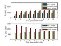
Fig. 12. Utilities of MSP and FSP versus spectrum bandwidth.
