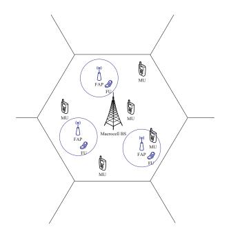
Fig. 1. The MSP and FSP coexistence Scenario.
