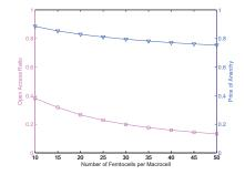
Fig. 5. Open access ratio of femtocell and POA versus femtocell density.
