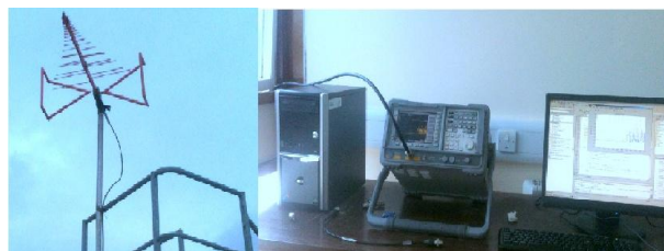
Fig 1. Measurement equipment employed in this study: Antenna, Spectrum Analyzer and Computer
