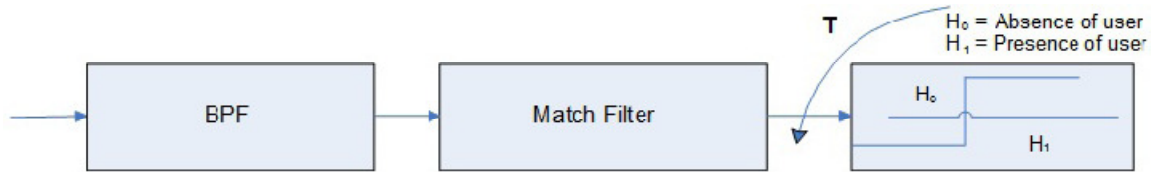
Figure 6: Block diagram of matched filter [1]
