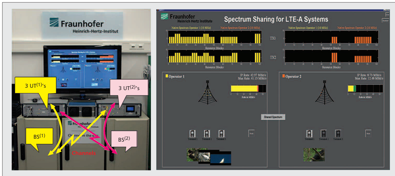
Figure 6. The LTE-advanced inter-operator orthogonal spectrum-sharing demonstrator.
