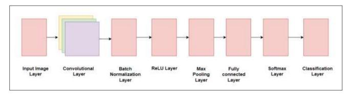
Fig 10. Layers of convolutional neural network
