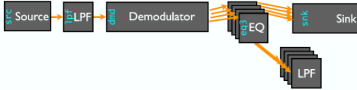
Figure 2: Software Radio with pipelined equalizer stage
