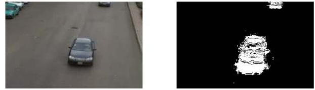
Fig. 2. Motion matrix sample, a: sample scene with two moving objects, b: the constructed motion matrix represents the pixels which are in motion in the current frame I_n .
