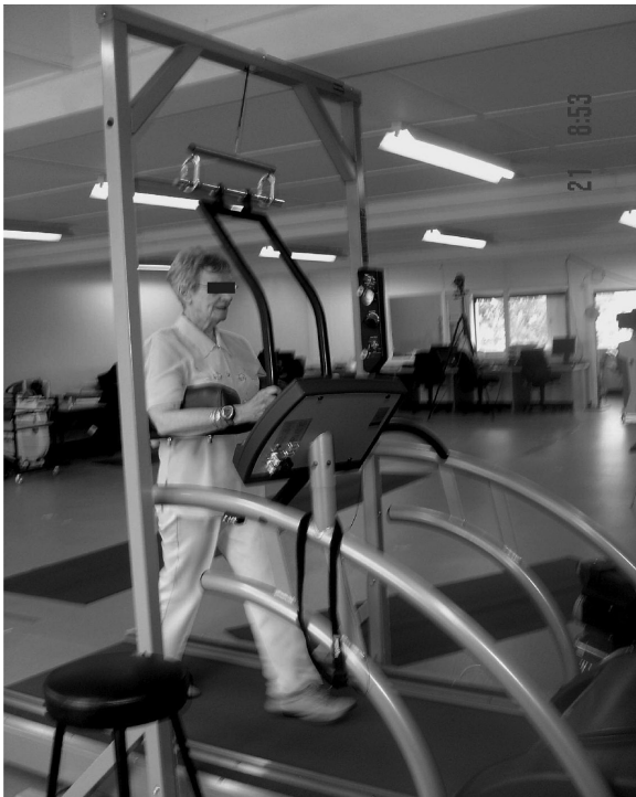
Fig. 1. A healthy older participant walking on a treadmill (Powerjog) with the pneumatic apparatus of body weight unloading (BWU) (Pneu-Lift, Pneumex) attached.
