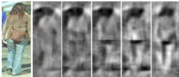
Figure 6. HOGgles visualizations of feature subsets. The first image on the left shows the target object in Sunny day . The rest of the images from left to right visualize 10%, 20%, 30%, 50%, and 100% feature usage, respectively.
