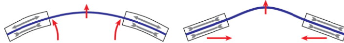
Figure 1. Illustration of lens curvature with one expanding and one contradicting piezo ring (bending mode, left) and both piezo rings contracting (buckling mode, right) [6].
