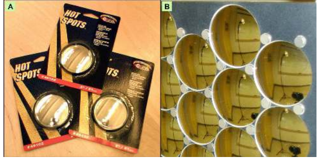
Figure 2: Spherical mirrors. (A) Adhesive-backed rear view mirrors used in the construction of the mirror array. (B) Detail of mirror array plate showing the steel pins that hold the mirrors in place.
