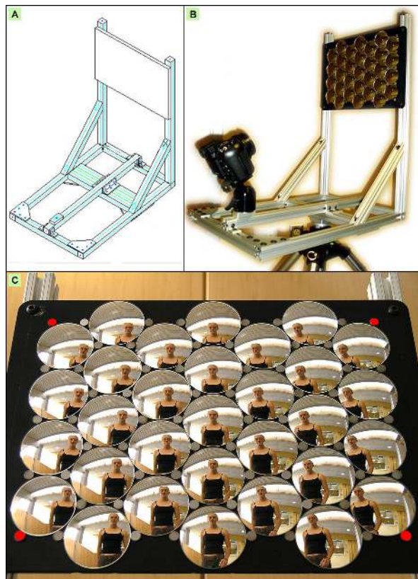
Figure 1: Spherical catadioptric array. (A) Mechanical design. (B) Constructed prototype. (C) Typical image captured by the 8 megapixel digital camera. The four corner pins marked in red are used to estimate the plate coordinate system (as discussed in Section 3).
