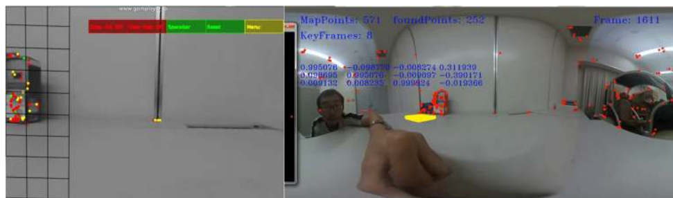
Figure 9. At the same position, PTAM fails to track as fewer feature points visible, while full-view SLAM tracks well.
