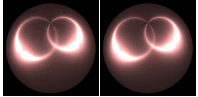
Figure 14: Results of an illumination simulation using the lifted Butterfly basis. A red, glossy, anisotropic sphere is illuminated by 2 area light sources. Left: solution with 2000 coefficients ( l_1 = 0.017 ). Right: solution with 5000 coefficients ( l_1 = 0.0035 )
