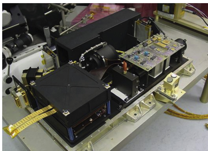
Fig. 1. SPICAV on a testbench without cover with the IR channel in front.
