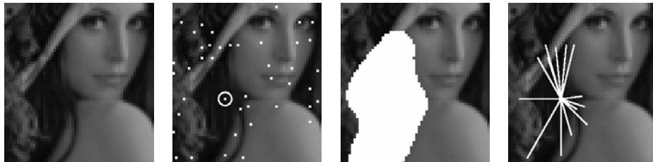
Fig. 1. An example of the determination of a spider. From left to right: 1) The original image (a part of the Lena image). 2) Interest points extracted with Lowe's scale space extrema operator are highlighted. A reliable point is marked, which is used as a salient point for the spider in the following. 3) A segment of pixels with a locally averaged brightness similar to the salient point is highlighted. Interest points in this area are used as the anchor points of the spider. 4) The final spider with 14 anchor points
