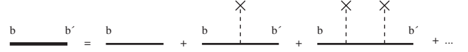
FIG. 3. Diagrammatic expansion for the Green's function when multiple scattering on the impurity site is considered. The solid line represents the full Green's function, and the thick line represents the noninteracting part of the Green's function. Each cross represents a scattering on an impurity site, and the dotted line stands for the impurity scattering potential. b and b' stand for band indices.
