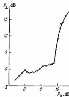
FIG. 4. Emission into the 'perpendicular' channel as function of pump power (YIG sphere,  $M \parallel \langle 100 \rangle$ ).
