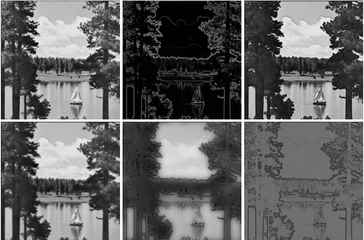
Fig. 2. Top: Grey-level image 'Lake' (Left) and its projection on the tangent bundle (Center) and the normal bundle (Right). Bottom: Diffusion of the Image 'Lake' at the times t = 0.0001 (Left), t = 0.01 (Center) and \lim_{t \rightarrow \infty} (Right).
