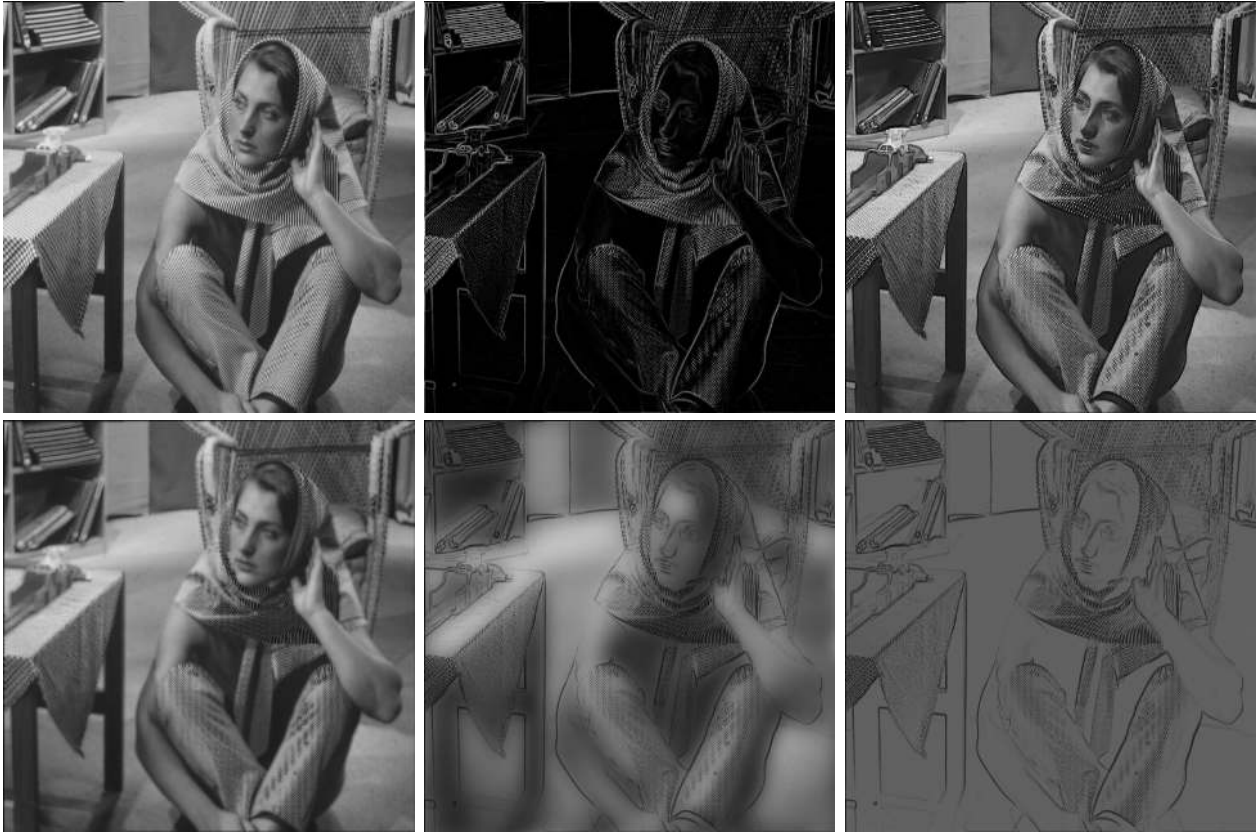
Fig. 1. Top: Grey-level image 'Barbara' (Left) and its projection on the tangent bundle (Center) and the normal bundle (Right). Bottom: Diffusion of the Image 'Barbara' at the times t = 0.0001 (Left), t = 0.01 (Center) and \lim_{t \rightarrow \infty} (Right).
