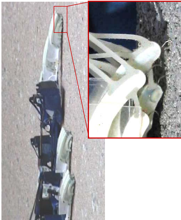
Fig.2 View of upper section of SpinybotII on concrete wall and detailed view of several spines independently engaging asperities on the concrete surface.
