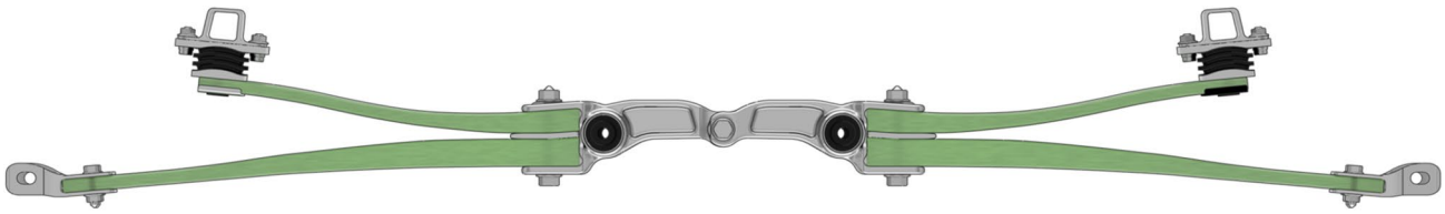
Fig. 1 Application example of glass fiber reinforced leaf springs in an automotive chassis assembly in order to achieve weight reduction (Kersten and Fiebig 2019)
