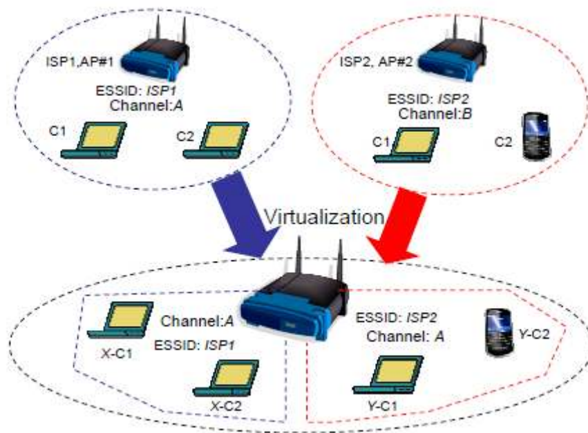
Figure 1: A single wireless access point emulating multiple virtual access points. Clients from different networks associate with corresponding VAPs though they use the same underlying hardware.
