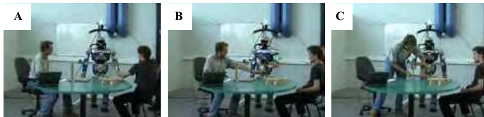
Fig. 2. Human-Robot cooperation in a furniture construction task. A. Robot takes a table leg from User2. B. Robot hands the leg to User1. C. Robot holds the table steady while User1 attaches the leg.
