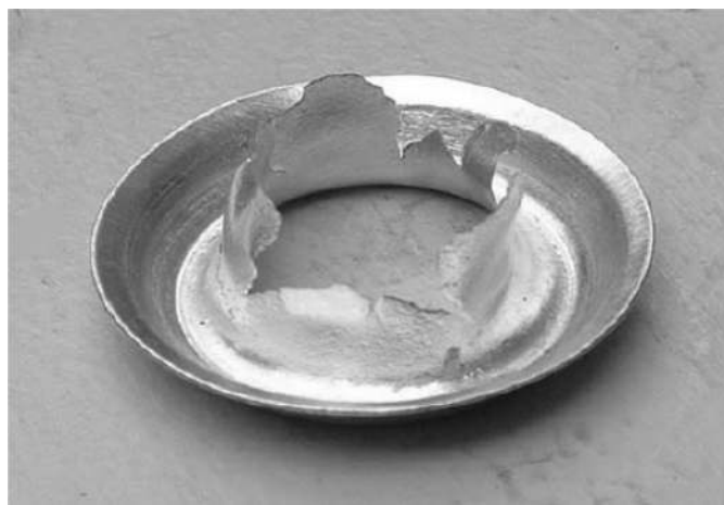
Figure 3. A ruptured Type B burst disk.
