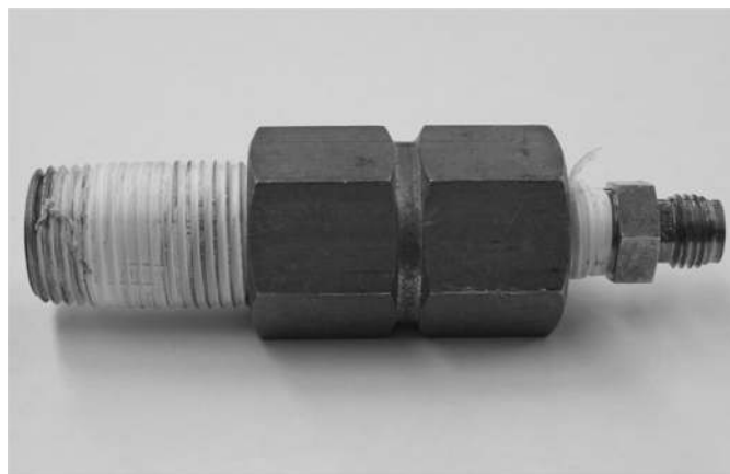
Figure 4. Downstream flow geometry used in initial experiments, composed of a 1/2" NPT pipe nipple 5.08 cm (2") long, a 1/2" to 3/8" NPT female brass reducing union, and 3/8" NPT male to 1/4" male Swagelok tube reducer.
