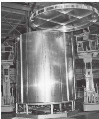
Figure 4. Environmental shroud assembly.
