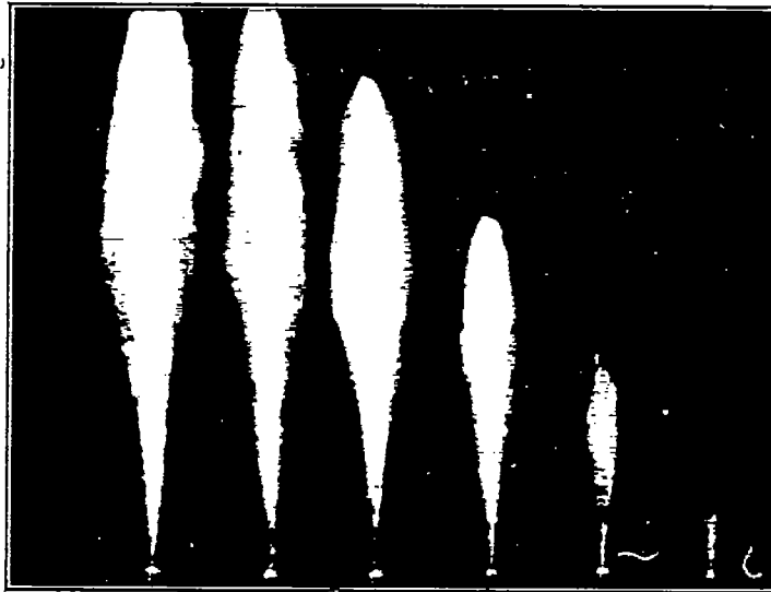
FIG. 3.—Injection pressure, 3,000 lb./sq. in. Chamber pressure, atmospheric
