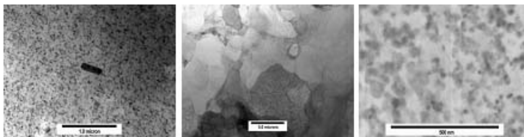
Figure 9: STEM photomicrographs of commercial 2124-T851 plate (left), as-spray-rolled 2124 (center), and spray-rolled 2124-T851 strip (right).
