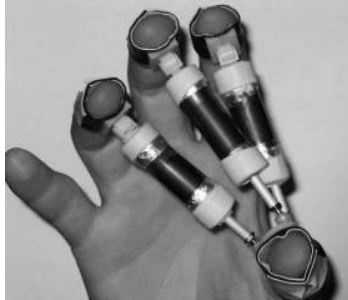
Figure 12. Prototype for the proposed force feedback concept with spring roll DE actuators.
