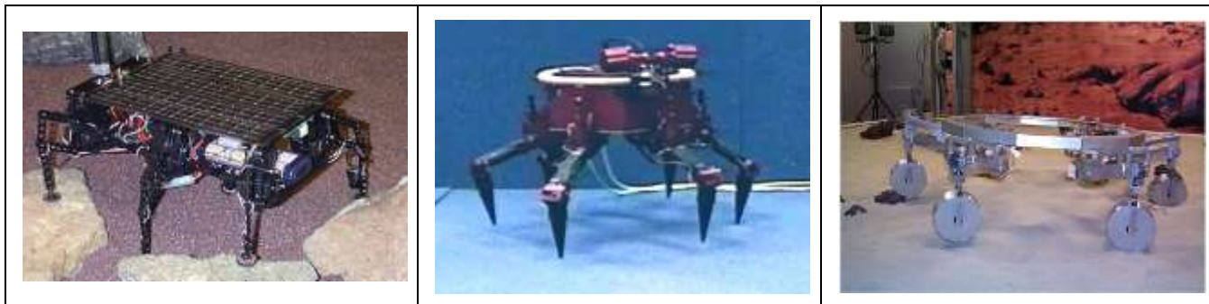
Figure 3-21 Several Generations of Hexapod Robots from the mid-1990s (Credit: NASA/JPL)
