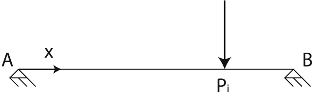
Fig. 3 An elastic rope supporting a load at a position x = X
